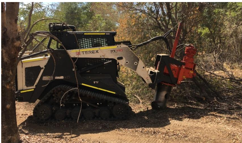
August 2018. Corer – removes the sandalwood stumps after we have cut the sandalwood trees down at the base. It can remove 120 stumps (cores) per hour. Each stump can contain up to 30% of the total oil in the tree.
